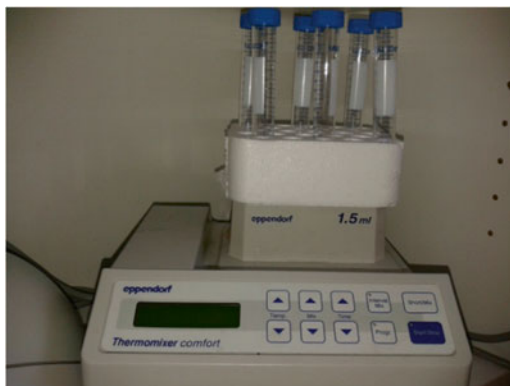
Fig. 4 A system to shake transformed bacteria. See text for further details
