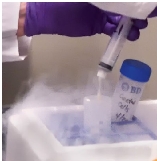
Fig. 2 Injection of pelleted human cells into liquid nitrogen to make “BB’s.” After centrifugation in a capped syringe, cells are injected into 50 mL conical tubes containing liquid nitrogen. Injection at a moderate rate prevents over-clumping of the cells. Use a pre-chilled spatula to break up any clumps
